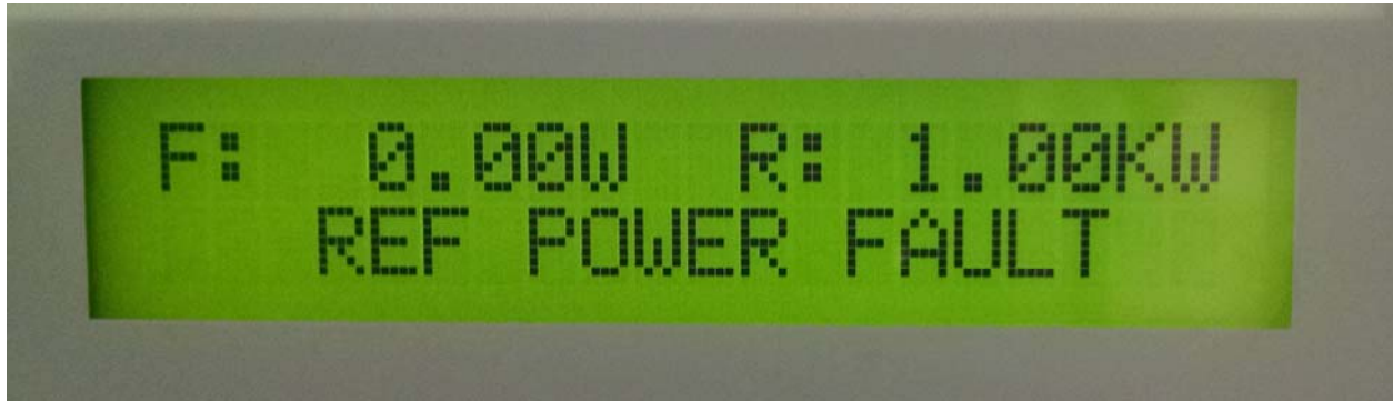
Fig. 4 Reflected Power Fault Indication
