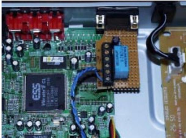
You can install the suggested circuit inside the player. Here we used a DB9 connector for connection and support. You can also use a 1/4" or 1/8" tip/ring/sleeve phone jack. Use the tip and ring for connections and the sleeve can be used for a ground between the player and CDS-302.
