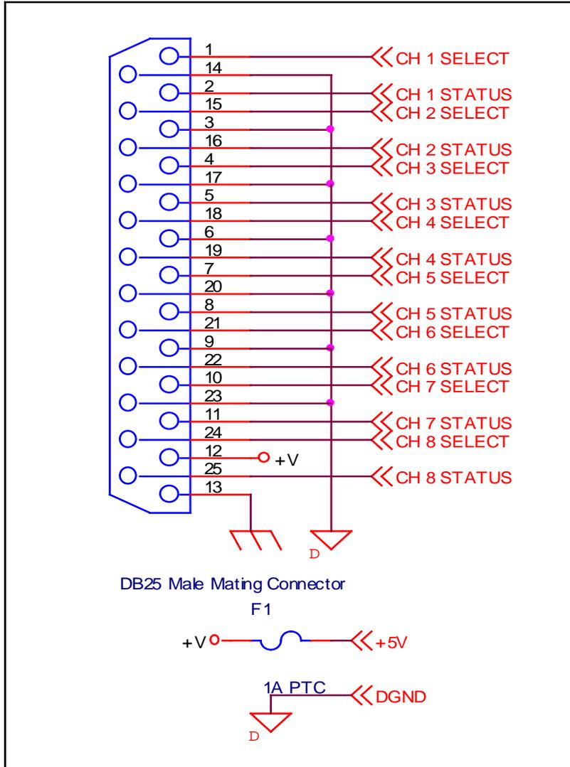
**Analog Input - Connector suggested wiring Table 3.**
