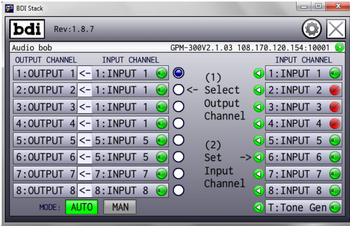
This screen shows a BDI model GPM-300 connected to the GUI.
