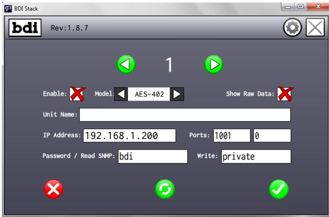
1. Select the device number at top by navigating the left and right arrows at the top of the screen.
