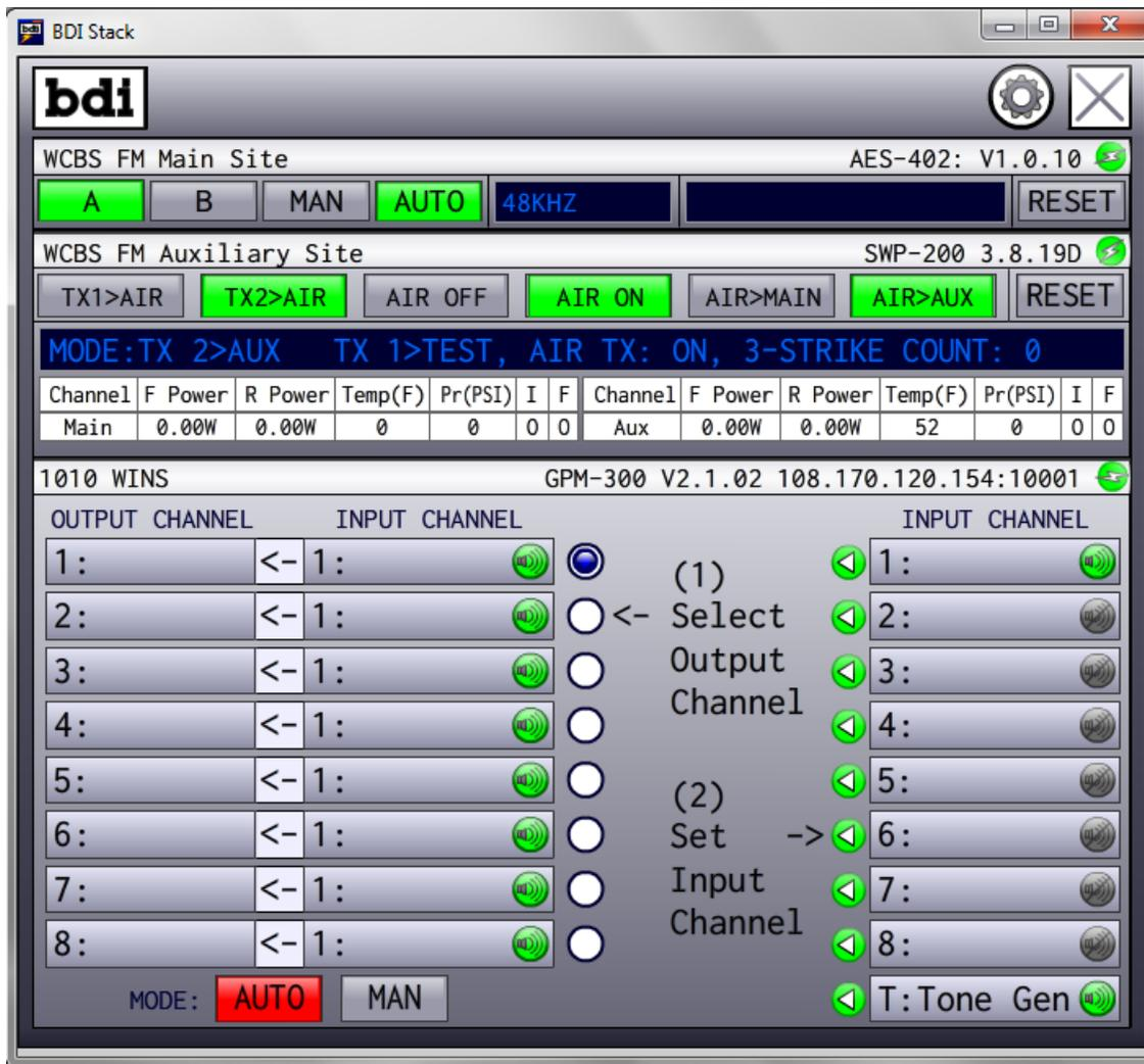
This screen shows three devices connected to the GUI, a BDI – AES-402 audio switcher, SWP-200 motorized switch controller, and a GPM-300 audio switcher.
